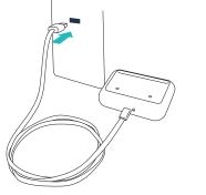
To charge the Battery Case use the micro-USB cable to plug into a power source. Battery case' life expectancy is 3 years or 1000 cycles of charging, whichever comes first.
